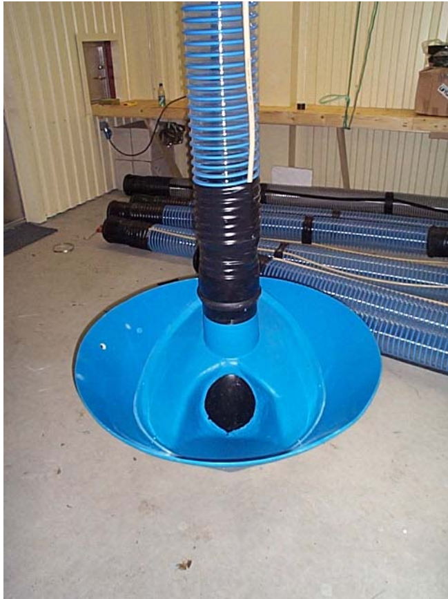
Figure 5. LiftUp® “china hat” suction unit showing intake, suction hose, and pressurized air line after retrieval at end of project.
