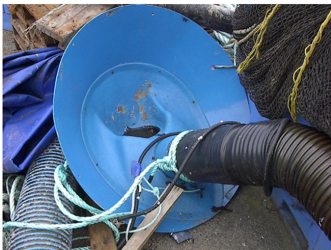
Figure 5. LiftUp® “china hat” suction unit showing intake, suction hose, and pressurized air line after retrieval at end of project.
